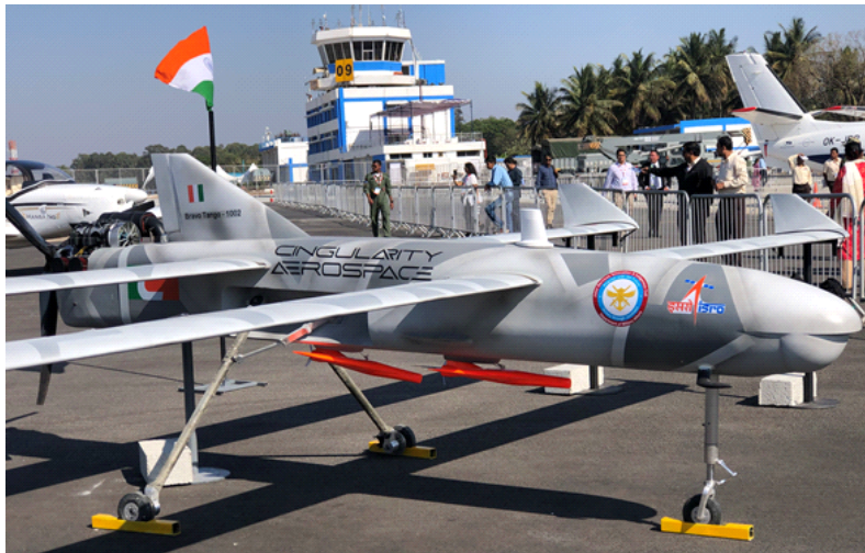
Fig 18. Tandem Wing Low Altitude Long Endurance Tactical UAV, courtesy Cingularity Aerospace
