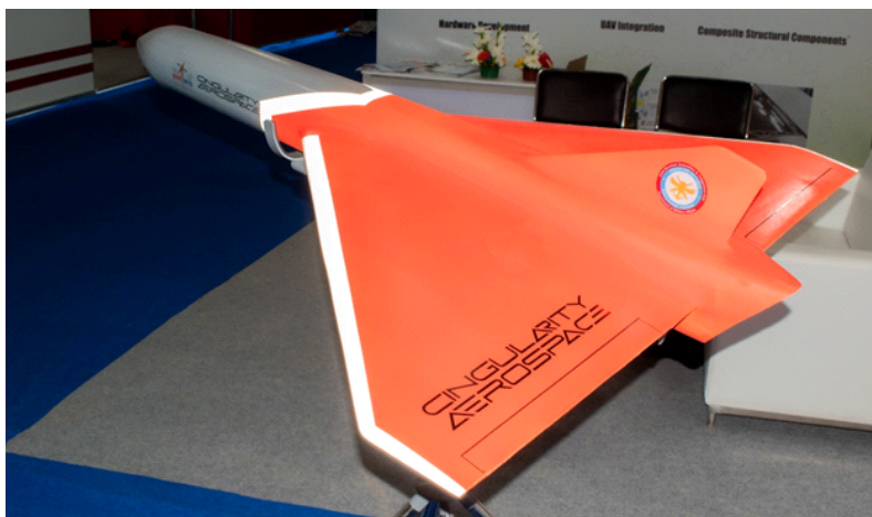
Fig 18A. Jet Engine High Speed Expandable Target Drone, courtesy, Cingularity Aerospace.
