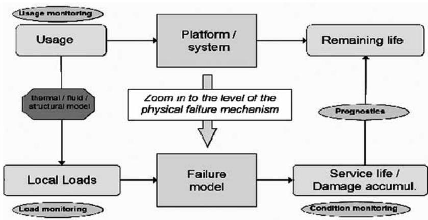
**Figure 1** Relationship between systems or component's utilisation, loads, and service life consumption.
