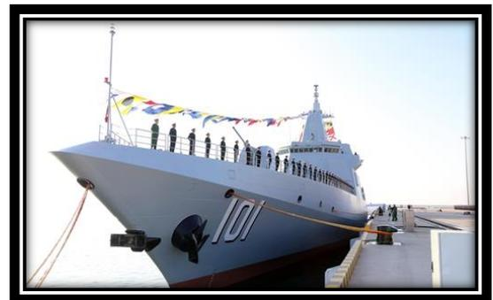
This is the first warship to enter Chinese naval service in 2020. Having a displacement of more than 10,000 tons, the Type 055 is a 180-metre-long and 20-metre-wide guided missile destroyer with 112 vertical launch missile cells capable of launching a combination of surface-to-air, anti-ship, land-attack and anti-submarine missiles.
