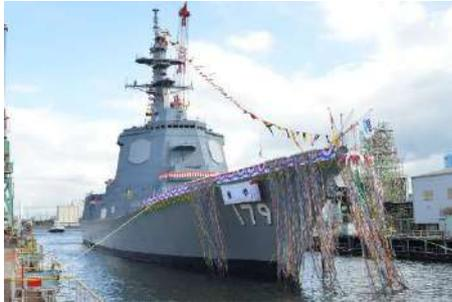
The Maya class of ships are 170 metres with a full load displacement of more than 10,000 tonnes. They are equipped with the US-developed Cooperative Engagement Capability (CEC) system, enabling them to share targeting data with other CEC-equipped ships and aircraft operating in the American and Australian navies. The Maya class also features the new Aegis system, and thus the ability to perform ballistic missile defence tasks.
