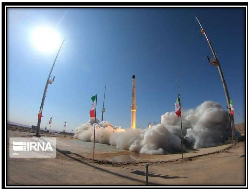
The *Zuljanah* is a three-stage rocket, with a solid-fuel engine in the first and second stages and a liquid-fuel engine in the third stage. It needs to complete a few more tests to become fully operational. When that happens, the SLV would be capable of launching satellites weighing up to 220 kilogrammes to an altitude of 500 kilometres above the earth's surface. It
