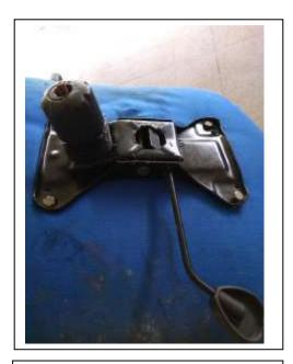
Revolving Chair swivel mechanism with base plate
